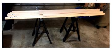
First load of lumber using 2"x2"x8 foot select pine for the frame and 3/4"x10"x8 foot solid oak boards for the top. The dimensions should match the speaker enclosures I built a few years ago. Weird working upside down but most of the joints are made using a Kreg tool...highly recommend for you woodworkers.
